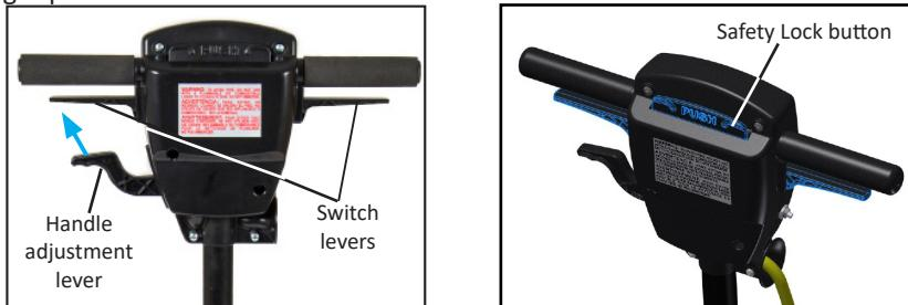
Once you have the handle height set to your preference and you are in the operators position, depress the handle slightly to elevate the pad from the floor. This is to avoid burning the floor on initial start up, before the operator is ready to move forward. Press in on the Safety Lock button with your thumbs and start the machine by depressing either the left, right or preferably both switch levers.
