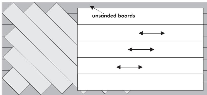
**Plank and Strip Floors** - sand in the direction the boards are laid, with the wood grain.
