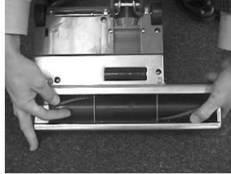
Inspect the brush assembly to remove the foreign object. Always unplug the vacuum before checking the brush. After the object is removed, turn on the vacuum as normal and continue cleaning.
