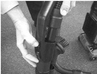
Check both the wand and hoses for blockage and remove any obstructions. A broom handle works well.
