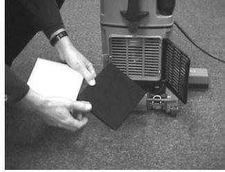
sponge filter it can be cleaned with detergent and water, then squeezed to remove the rinse water. Allow it to dry before putting it back in. However, if the filter is torn or excessively worn it should be replaced. **White Hepa Filter:** In order to obtain the optimal performance from a hepa filter, it should not be cleaned and used again. When dirty, replace it. The average life of a filter depends on the environment and the visible layering of debris.
