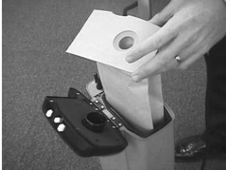
Be sure that the metal sensor prong is not showing when the bag is installed.
