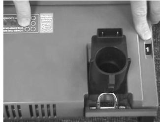
Remove the three screws to allow the vacuum plate to lift up showing the brush assembly.
