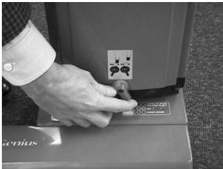
Then look into the swivel throat assembly by depressing the foot pedal and remove the obstruction.
