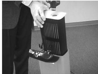
Remove and shake or vacuum the filter. If it is worn or uncleanable, replace it.
