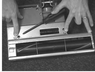
Pull the brush out of the machine on the extended end shown and remove the end cap. Slide out the worn brush strips and replace. Reattach the end cap and vacuum plate.
